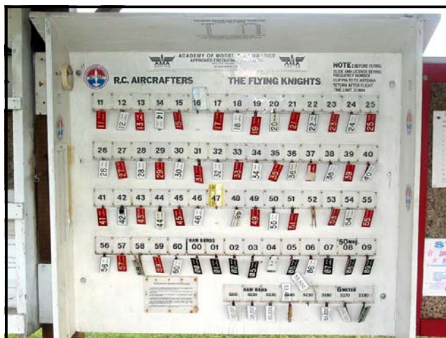
This tag board is used to ensure that RC aircraft fliers don't use a radio frequency already in use at the field.
