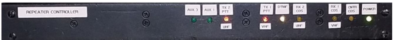
Figure 6 Repeater Controller (Front View)
