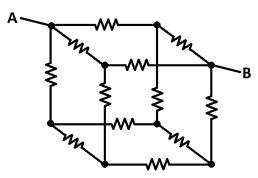
Each resistor in the cube is 60 ohms.
