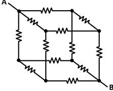
Each resistor in the cube is 30 ohms.
