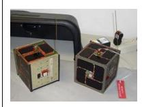
this mission, however, BEVO-1 and AggieSat2 launched as one unit and then separated to collect position data and test a new NASA Global Positioning System receiver known as DRAGON.
