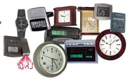
clock actually has a miniature radio receiver inside. In the US, the radio-controlled clocks receive signals from NIST radio station WWVB, located near Fort Collins, Colorado.
