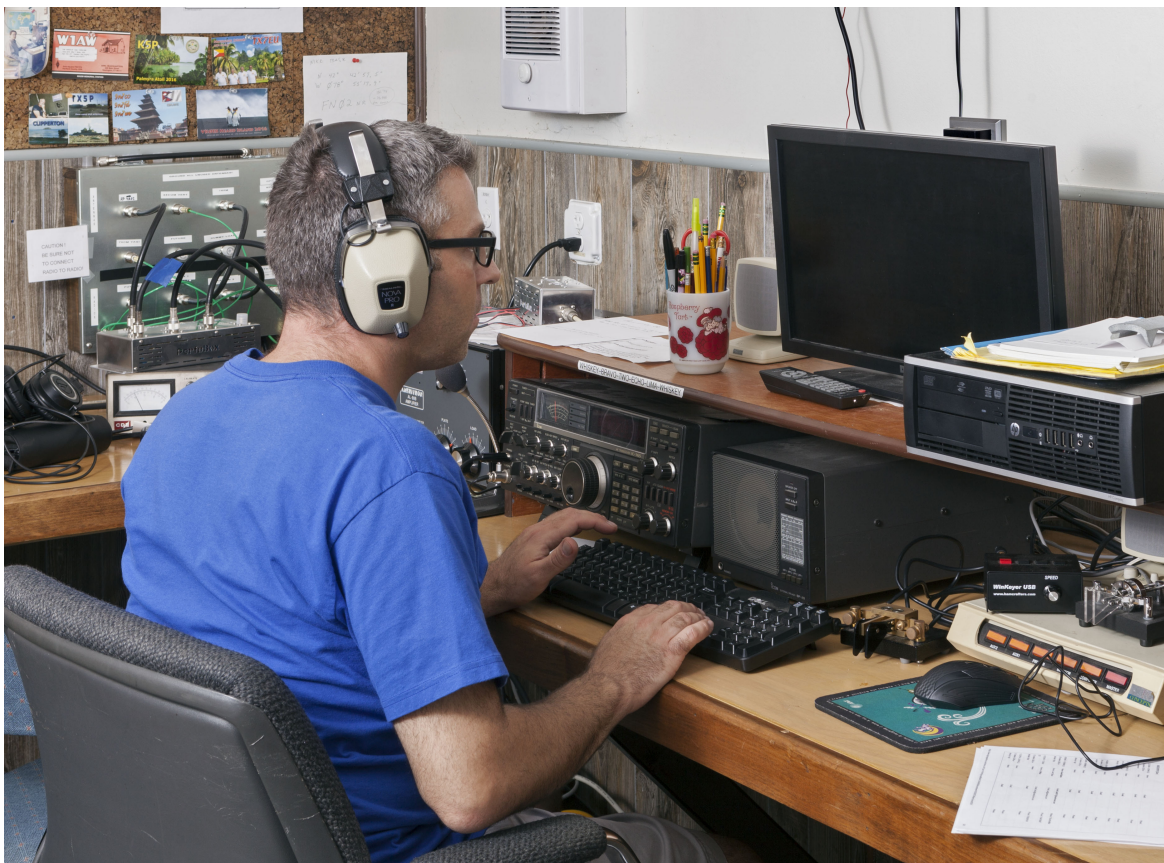
Scott KB2KOL at one of the CW stations. Just above Scott's left shoulder you can see the combiner that allowed radios on 15, 20 and 40 meters to operate simultaneously with the HF beam antenna. It also has a port for 10 meters.
